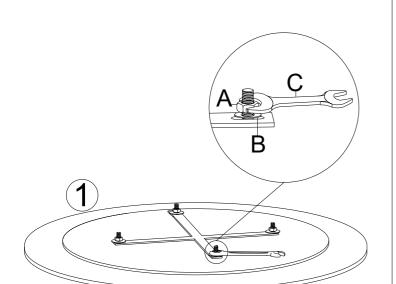
Remove the hex nut and washer, as shown in image view.
