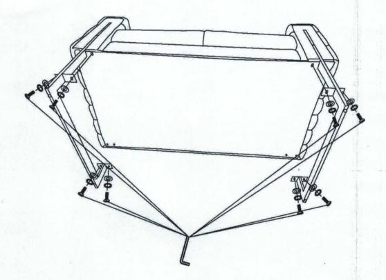
Insert the metal leg into the gap and tighten the hardware with a wrench
