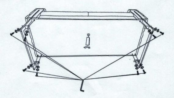
Insert the metal leg into the gap and tighten the hardware with a wrench
