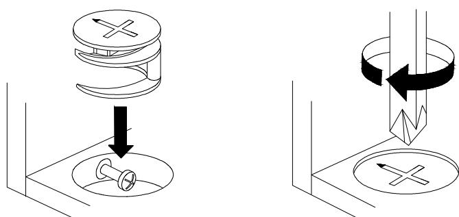
Turn cam lock clockwise to tighten.
