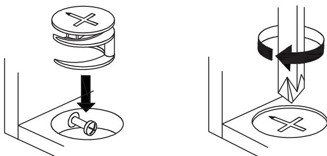
Turn cam lock clockwise to tighten.
