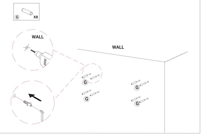
Step 11 Next, measure where you want to mount on your wall, drill the holes, hammer in the anchors (G) and then screw the mounting equipment (E) into the wall using 4 screws (F) each.
