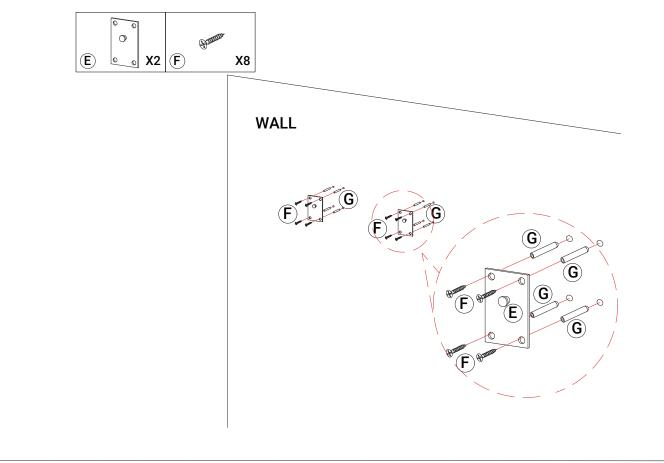
$\label{eq:step12} Step 12 \ | \ {\sf Finally, align the mounting brackets and hang on your wall.}$
