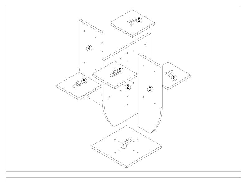
Step 1 Let's get started. Start by attaching board 3 to board 2 by first placing 2 wooden dowels (C) in the inner holes of board 3, then aligning in place and securing with 2 wooden hex screws (D).
