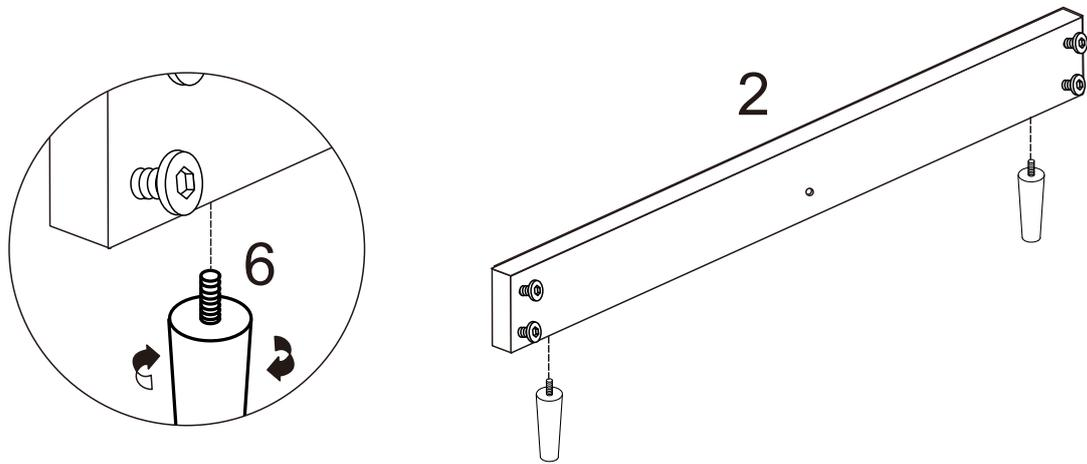
Step2 Please install part (2) and (3) on part (4) and tighten the blots (H1)
