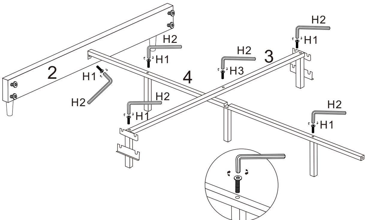
Step3 Lay the headboard (1) flat on the clean floor, put the headboard support frame (8) on it, and tighten it with (H1) and (H2)
