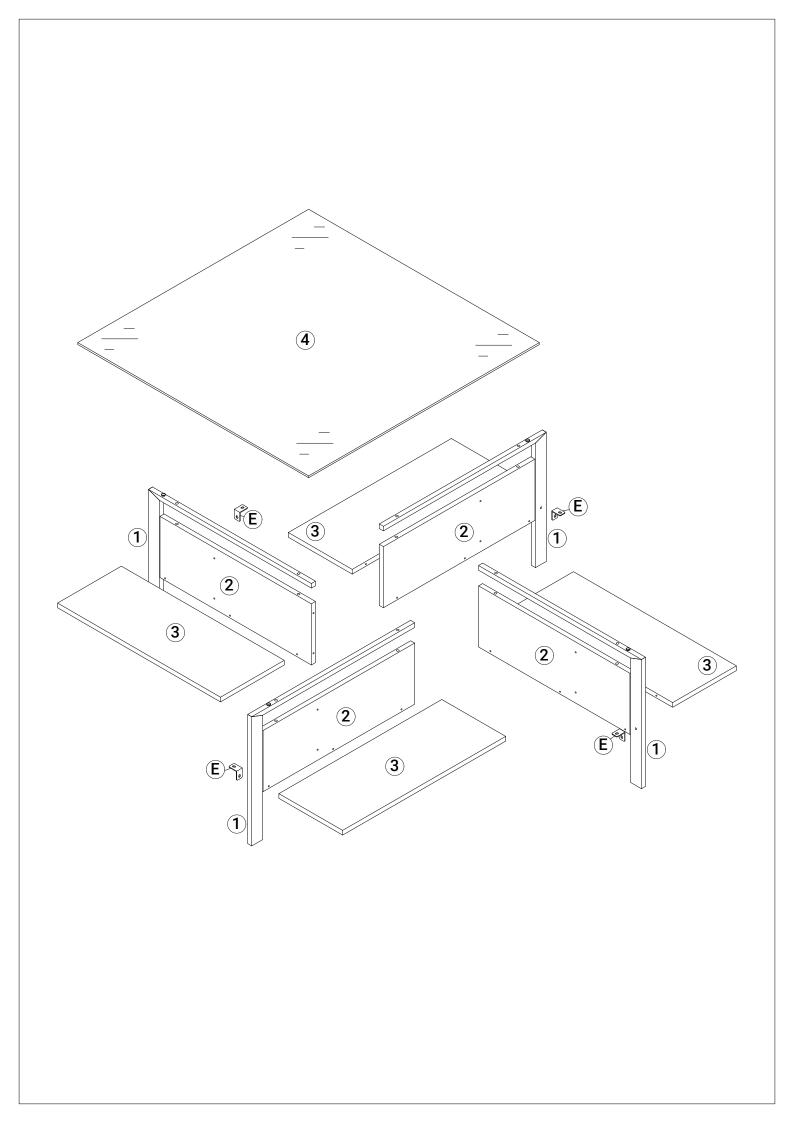
Step 1 Lets get started. Start by attaching the feet (C) to the support frames (1) and then add the brackets (E) to each frame using 1 bolt (A). Pay attention that the brackets are facing upward, in an upside down L position.
